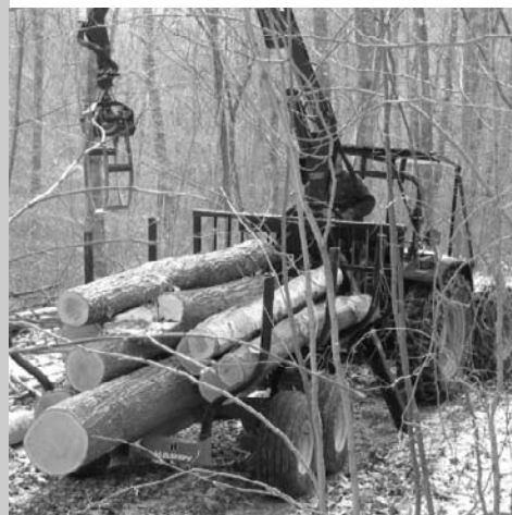
Bill Torrey's log forwarder helps minimize soil compaction and erosion during logging at the Little Hogback Community Forest.
