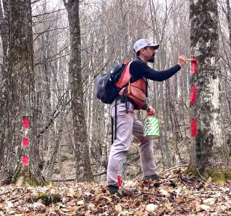
Left: VFF Conservation Forester Ralph Tursini refreshes boundary paint on witness trees near a corner post. While only licensed surveyors create boundary markings, landowners can and should regularly refresh those survey markings to keep them visible. We offer landowners detailed instructions how to do that themselves. If they prefer to hire out the work, Ralph steps in as needed.
